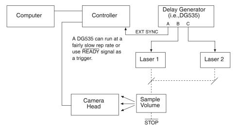
Figure 55. Setup for IEC Eexperiment with Two Lasers
